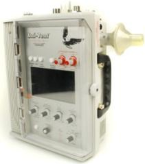
**CAUTION:** Routine use of an external filter (Impact p/n 465-0024-00 or equivalent) will prevent entrainment of particulate and increase the service life of the flow transducers.
